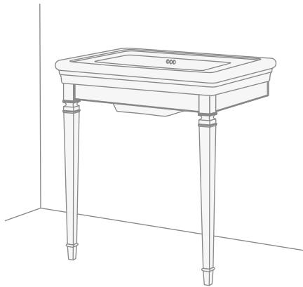
**14)** Seal the area between the basin and the wall with silicone.
