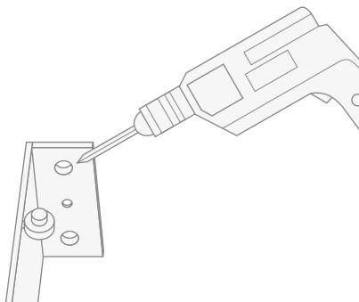
*Insert the rawl plugs which are not supplied in the holes, position the structure again and fasten it using screws which are not supplied.*
