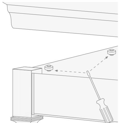
*If necessary, work on the adjustable supports using the screwdriver.*
