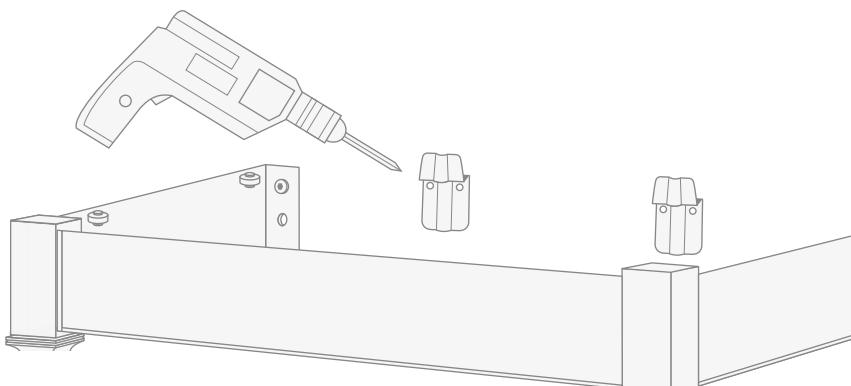
*Mount the basin support brackets, fastening them with screws and rawlplugs (not supplied).*
