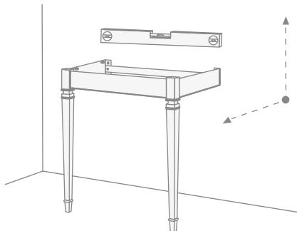
*Use a level to check that the structure is positioned correctly in both a parallel and perpendicular position to the wall.*
