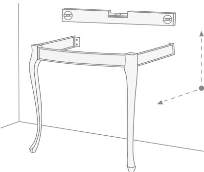
Use a level to check that the structure is positioned correctly in both a parallel and perpendicular position to the wall.
