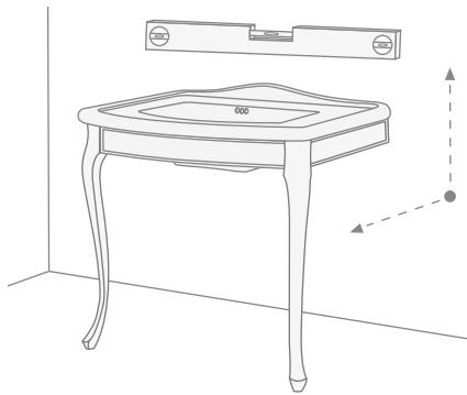
**9)** If necessary work on the adjustable supports to obtain a better result.
