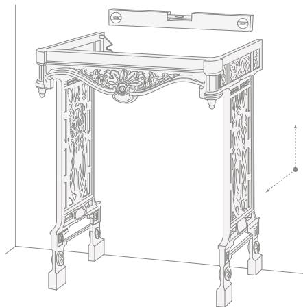
**6)** Mount the adjustable supports for the basin (D), screwing them into the slots in the metal structure.
