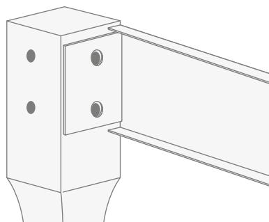
**3)** Fasten the side supports to the legs using the socket-head screws and washers supplied.
