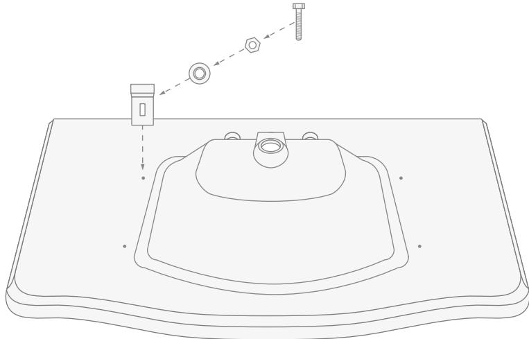
**11)** Tighten the 4 screws and 4 nuts locking the basin on the marble top.
