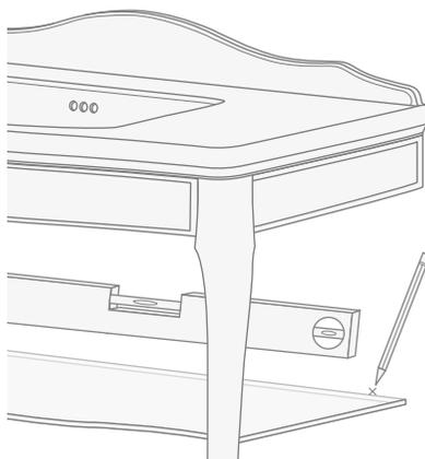
**14)** Remove the shelf, drill the holes for the supports on the wall and mount the supports with the fastening screws faced downwards.
